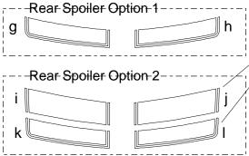
Option 2 Rear Spoiler Top pieces splice/overlap approximately .125" (3.17mm) over Rear Spoiler Rear pieces just after the edge of the Factory Spoiler at time of installation.
