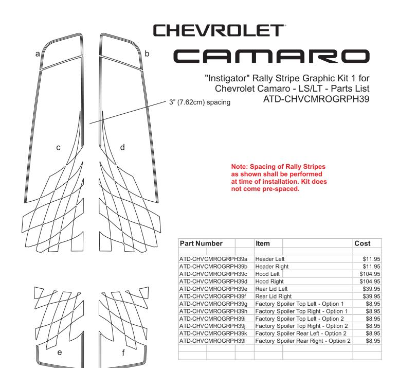
Option 2 Rear Spoiler Top pieces splice/overlap approximately .125" (3.17mm) over Rear Spoiler Rear pieces just after the edge of the Factory Spoiler at time of installation. Thus, we suggest the installation of the Rear Spailer Rear pieces prior to the application of
