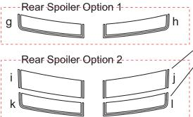
Option 2 Rear Spoiler Top pieces splice/overlap approximately .125" (3.17mm) over Rear Spoiler Rear pieces just after the edge of the Factory Spoiler at time of installation.
