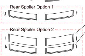
Option 2 Rear Spoiler Top pieces splice/overlap approximately .125" (3.17mm) over Rear Spoiler Rear pieces just after the edge of the Factory Spoiler at time of installation.
