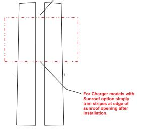
Set 4" (101.60mm) spacing at time of installation
