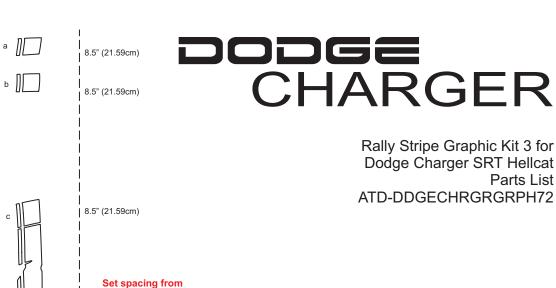
side of stripe to Centerline of vehicle with distances shown at time of installation 9.5" (24.13cm) 9.5" (24.13cm) **Vehicle** Centerline 10" (25.40cm) 10.375" (26.35cm) 11" (27.94cm) 11" (27.94cm) 11" (27.94cm) 11" (27.94cm)
