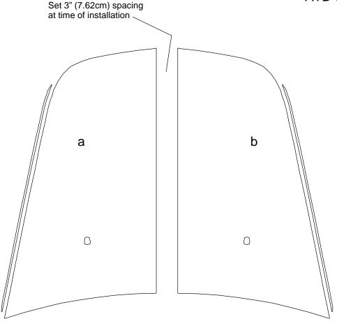
Note: Spacing of Stripes as shown shall be performed at time of installation. Kit does not come pre-spaced.
