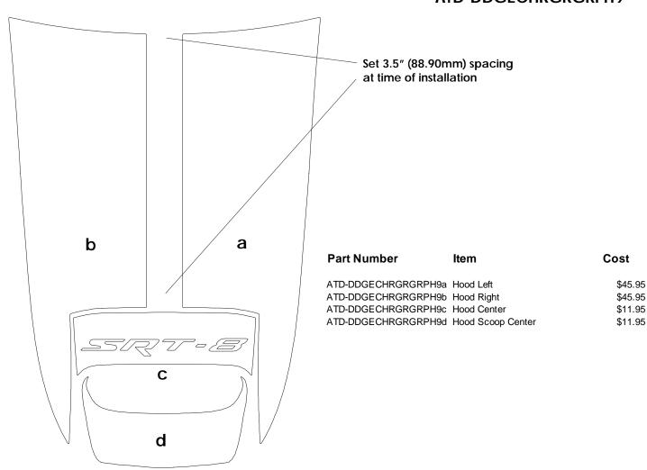
Note: Spacing of Rally Stripes as shown shall be performed at time of installation. Kit does not come pre-spaced.
