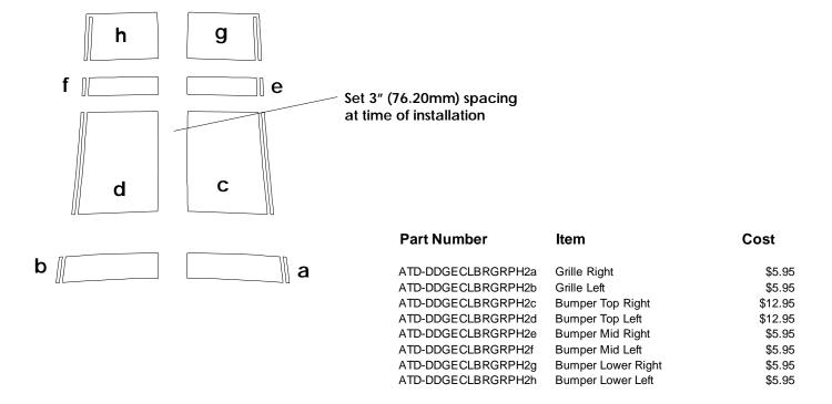
Note: Spacing of Rally Stripes as shown shall be performed at time of installation. Kit does not come pre-spaced.
