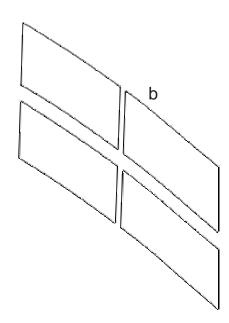
Stripe is designed to set 1.25" (31.75mm) from front door jamb and along the Challenger's distinct body side line. We suggest dryfitting the piece to become familiar with placement.
