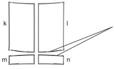
Due to the difficulty of installing one (1) piece stripes on the Rear Lid, two (2) piece spliceable sets are provided. Rear Lid Top and Rear Lid Rear pieces, respectively, are designed to splice/overlap approximately 0.2" (5.08mm) after the Rear Lid Rear piece is applied.
