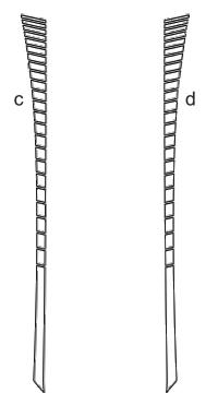
Note: Spacing of Stripes as shown shall be performed at time of installation. Kit does not come pre-spaced. Stripe kit is set to be installed just above the Dakota's distinct body side line and Hood edge Dryfitting graphic is recommended to become familiar with correct placement.
