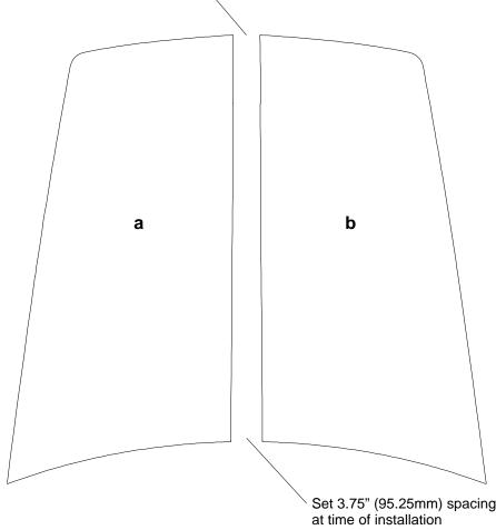
Note: Spacing of Hood pieces shown shall be performed at time of installation. Kit does not come pre-spaced. Removal and reinstallation of Windshield Washer Nozzles is suggested for ease of installation.
