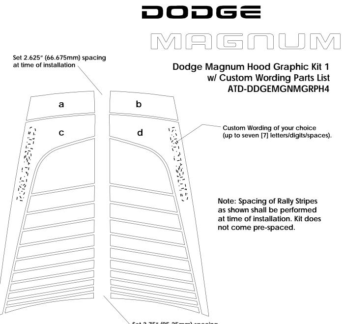
Set 3.75" (95.25mm) spacing at time of installation
