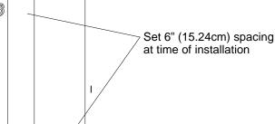
Note: Spacing of Rally Stripes as shown shall be performed at time of installation. Kit does not come pre-spaced.
