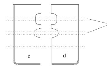
Installation Tip: Take care NOT to "bridge" the depressions found on the tailgate. Carefully work the pieces into and out of the depressed areas as the graphic is applied.
