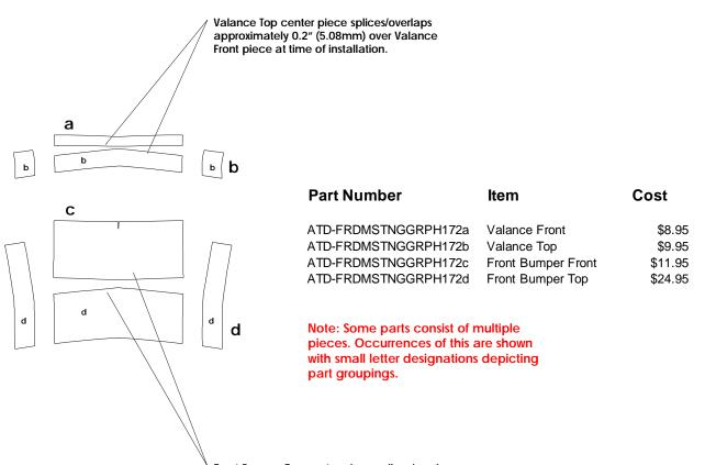
Front Bumper Top center piece splices/overlaps approximately 0.2" (5.08mm) over Front Bumper Front piece at time of installation.
