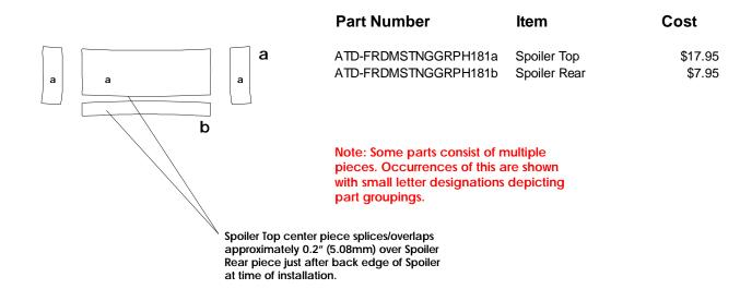
Note: Spacing of Rally Stripes as shown shall be performed at time of installation. Kit does not come pre-spaced.
