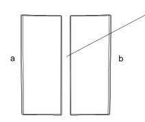
Set 0.875" (22.225mm) spacing at time of installation
