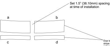
Due to the difficulty of installing a one (1) piece stripe on the Rear Spoiler, a two (2) piece spliceable set is provided. The Spoiler Top and Spoiler Rear pieces, respectively, are designed to splice/overlap approximately 0.2" (5.08mm) after the Spoiler Rear piece is applied.
