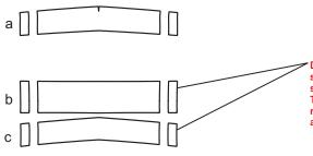
Due to the difficulty of installing a one (1) piece stripe on the Front Bumper, a two (2) piece spliceable set is provided. The Front Bumper Top and Front Bumper Front pieces, respectively, are designed to splice/overlap approximately 0.2" (5.08mm).
