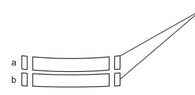
Due to the difficulty of installing a one (1) piece stripe on the Rear Bumper, a two (2) piece spliceable set is provided. The Rear Bumper Top and Rear Bumper Rear pieces, respectively, are designed to splice/overlap approximately 0.2" (5.08mm).
