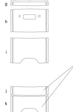
Due to the difficulty of installing a one piece stripe on the Rear Bumper, a one (1) piece stripe and an optional two (2) piece spliceable set is provided.
