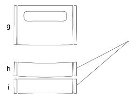
Due to the difficulty of installing a one piece stripe on the Rear Bumper, a two (2) piece spliceable set is provided. The Rear Bumper Top piece splices/overlaps approximately 0.2" (5.08mm) over the Rear Bumper Rear piece at time of installation.
