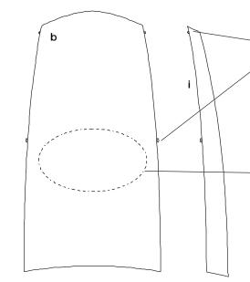
Note:Ovalsatsideofgraphics serve as registration dots for ease of installation. Center graphics should be placed and setfirst.Highlightpiecescan thenbesetaccordingtothe registrationdots.
