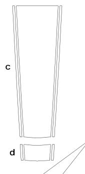
Note: Spacing of Rally Stripes as shown shall be performed at time of installation. Kit does not come pre-spaced.
