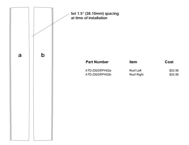
Note: Spacing of Rally Stripes as shown shall be performed at time of installation. Kit does not come pre-spaced.
