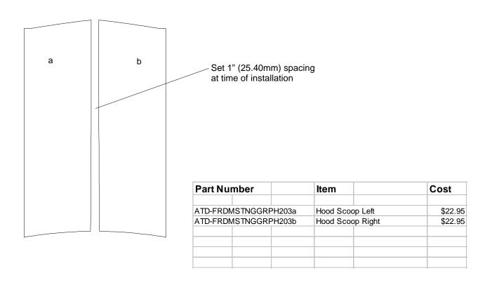
Note: Spacing of Rally Stripes as shown shall be performed at time of installation. Kit does not come pre-spaced.
