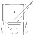
Due to the difficulty of installing a one (1) piece stripe on the Rear Lid, a two (2) piece spliceable set is provided.
