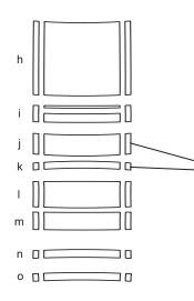
Due to the difficulty of installing a one (1) piece stripe on the factory Rear Spoiler, a two (2) piece spliceable set is provided. The Rear Spoiler Top and Rear Spoiler Rear pieces, respectively, are designed to splice/overlap approximately 0.2" (5.08mm). We suggest applying the Rear Spoiler Rear piece first.
