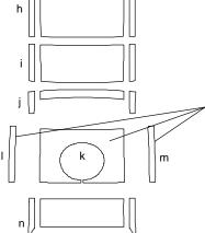
Due to the difficulty of installing a one (1) piece stripe on the Rear Lid Rear, we recommend installing the trim pieces separately after successful installation of the Rear Lid Rear piece.
