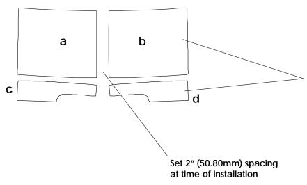
Rear Spoiler Top pieces splice/overlap approximately.125" (3.175mm) over Rear Spoiler Rearpiecesjustafter backedge of RearSpoilerat time of installation.
