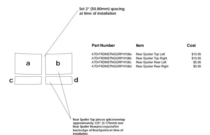
Note: Spacing of Rally Stripes as shown shall be performed at time of installation. Kit does not come pre-spaced.
