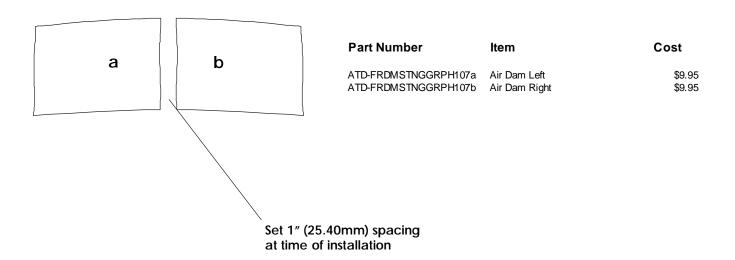
Note: Spacing of Rally Stripes as shown shall be performed at time of installation. Kit does not come pre-spaced.
