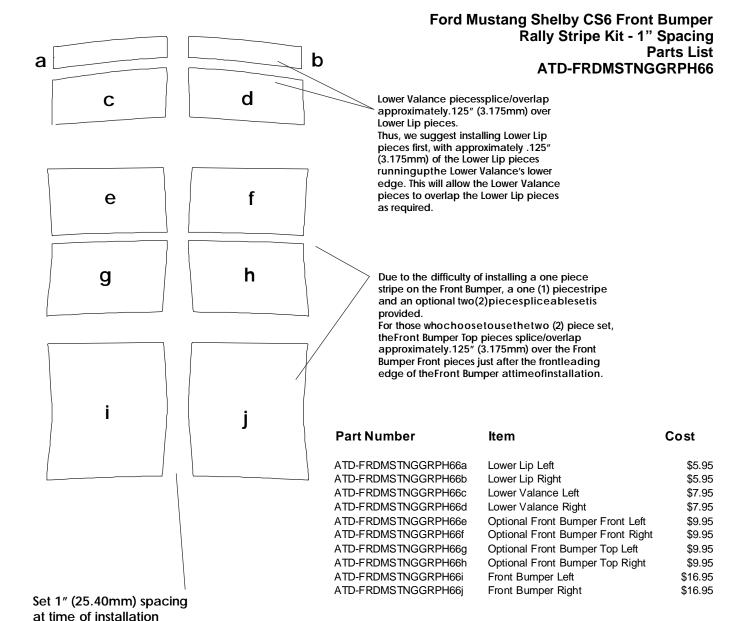
Note: Spacing of Rally Stripes as shown shall be performed at time of installation. Kit does not come pre-spaced.
