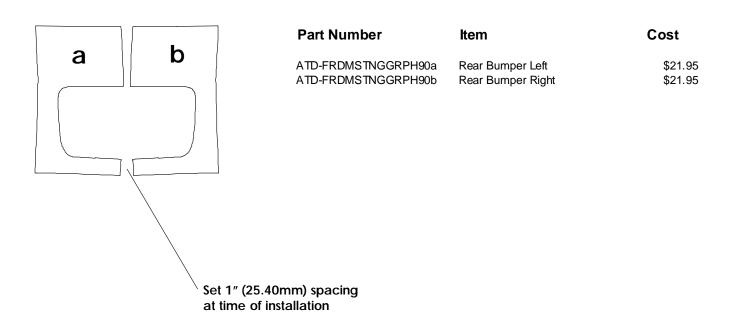
Note: Spacing of Rally Stripes as shown shall be performed at time of installation. Kit does not come pre-spaced.
