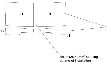
Rear Spoiler Top pieces splice/overlap approximately.125" (3.175mm) over Rear Spoiler Rearpiecesjustafter backedge of RearSpoilerat time of installation.
