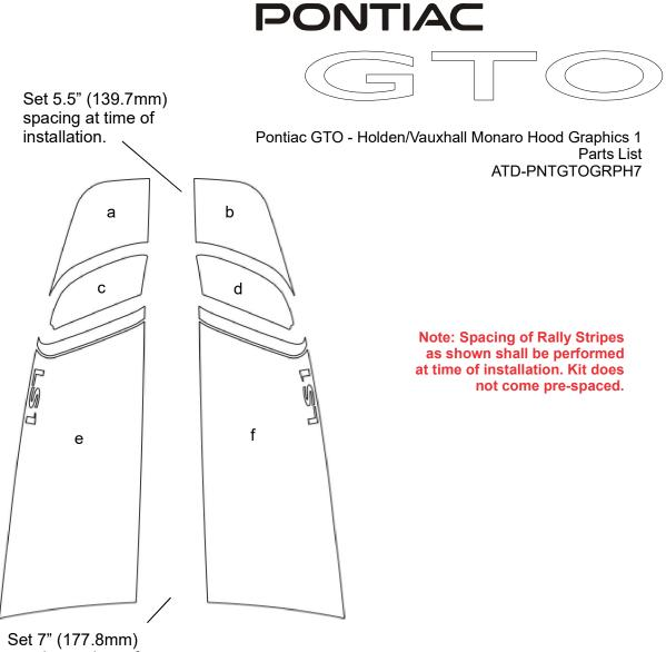
Set 7" (177.8mm) spacing at time of installation.
